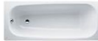
LAUFEN PRO Bathtub, drop-in version, enamelled steel (3.5 mm) / with holes for handles pre-drilled 1700 x 700 mm H224950 / H224953
