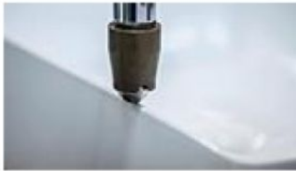
THE THIN-WALLED SAPHIRKERAMIK WAS TESTED FOR IMPACT RESISTANCE AT THE KERAMIK INSTITUT MEISSEN
