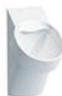
Siphonic urinal ,rimless', internal water inlet, without mounting holes for cover, with electronic control system, mains operated (230V), with integrated blue-tooth, vandalproof
